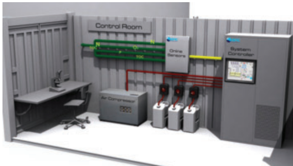
Automated Control System: the figure to the right illustrates the automated control and online monitoring system.
